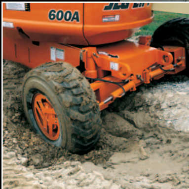
Oscillating Axle for Tough Terrain
