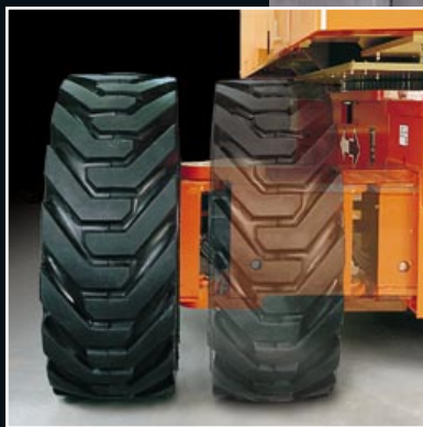
Pin-less Axle Extension for Faster Setup
