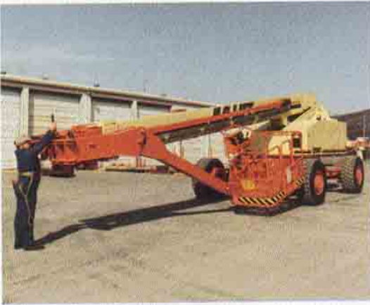
The fly boom tip can be swung around and pinned to reduce transport length.
