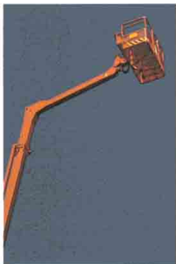
13 ft. (4m) Extend-A-Reach feature increases operator versatility in positioning the work platform.
