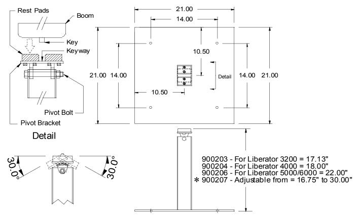
\*NOTE: Adjustable Boom Rest requires welding the telescopic sections together at the custom height. For this reason, adjustable Boom Rest is shipped prime painted.
