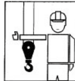
RAISE BOOM - With arm extended, fingers closed, thumb pointing upward.
