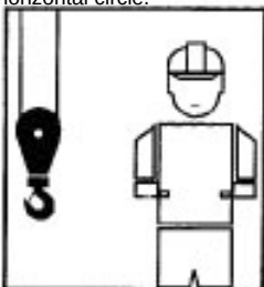
RETRACT BOOM - (Telescopic Booms) Both fists in front of body with thumbs pointing inward.
