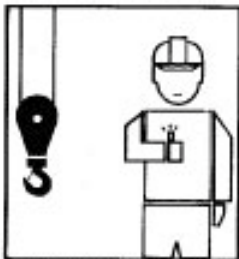
EXTEND BOOM - (Telescopic Booms) One Hand Signal. One fist in front of chest with thumb tapping chest.
