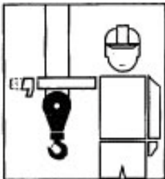
LOWER BOOM - RAISE LOAD Arm extended, thumb pointing down, flex fingers in and out until desired movement is completed.
