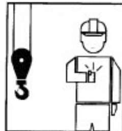
RETRACT BOOM - (Telescopic Booms) - One Hand Signal. One fist in front of chest, thumb pointing outward and heel of fist tapping chest.
