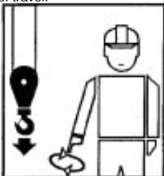
LOWER - With arm extended downward, forefinger pointing down, move hand in small horizontal circle.
