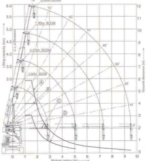
"Working radius" means a horizontal distance from the center line of rotation to the hook center. Working radius shown actual radius which considered deformation by lifted load
