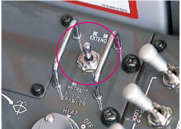
Side frame extend/retract switch
