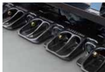
High-durability box type track shoes Lower rollers with 20% greater contact width
