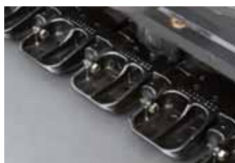
High-durability box-type track shoes
