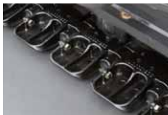
High-durability box-type track shoes
