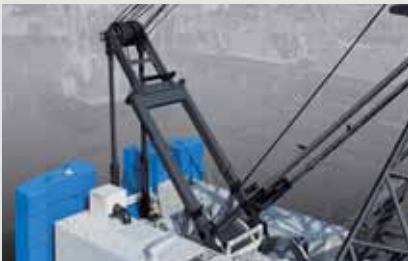
Folding gantry with hoisting cylinder
