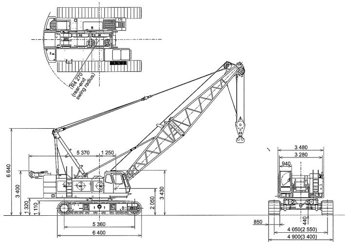
Notes: 1. Dimensions shown in ( ) are with side frames fully retracted.
