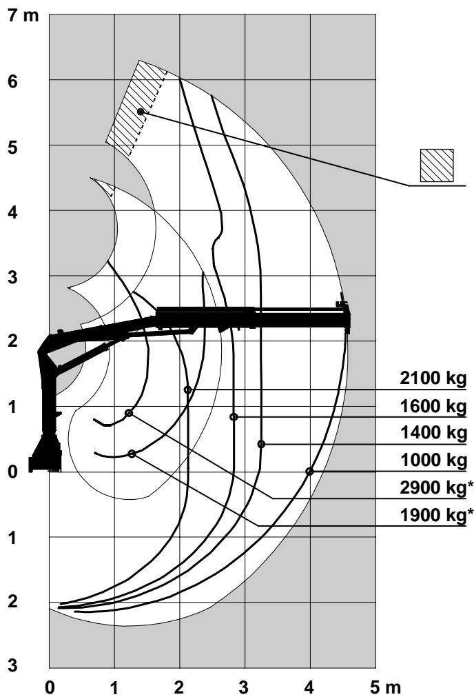
Extra working-area for crane without built in load holding valve
