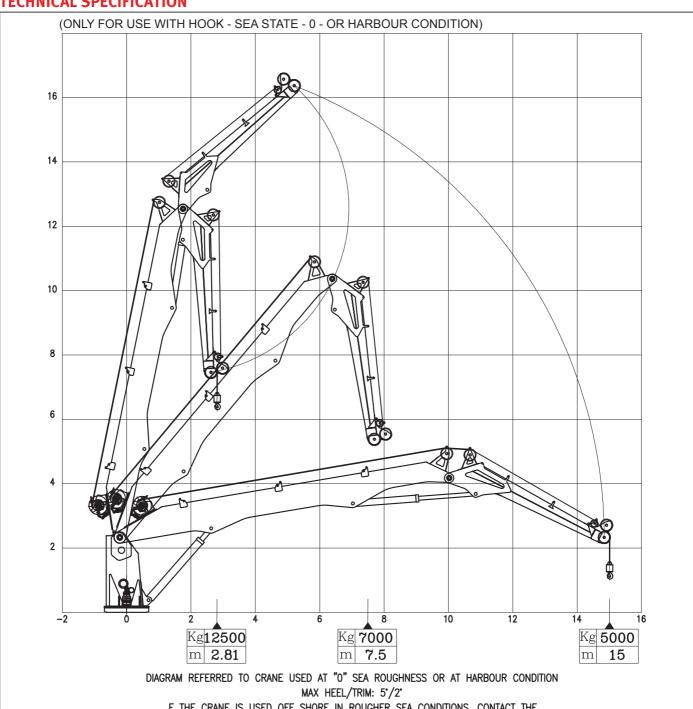
F THE CRANE IS USED OFF SHORE IN ROUGHER SEA CONDITIONS, CONTACT THE MANUFACTURER TO ESTABILISH LOADING CAPACITIES OR REDUCTION PARAMETERS.
