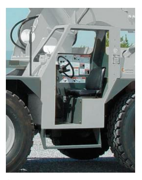
Standard: Open air cab shell w/overhead safety
