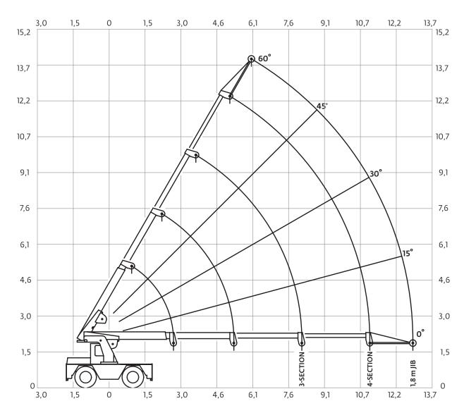
Operating radius in meters from axis of rotation
