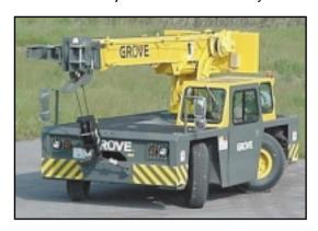
Full power standard 24 ft. (7 m) boom with 10 - 16 ft. (3 - 5 m) fixed or 45 degree offsettable telescopic boom extension that gives max tip height of 38 ft. (11.5 m) or 44 ft. (13 m) respectively
