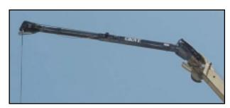
Low-profile quick reeve boom nose design with single metallic sheave for improved accessibility
