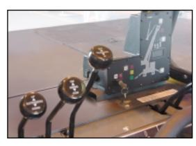
Interactive PAT/LMI system with actual load display that provides visual prewarning at 90% of rated capacity
