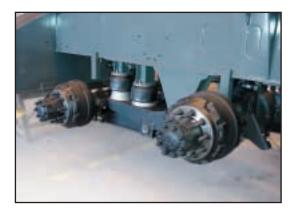
Standard front and rear air ride suspension provides comfortable ride at max speed of 65 mph
