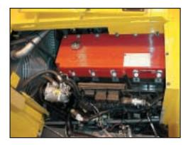
Electronically controlled Cummins six cylinder, turbo charged, 400 bhp diesel -- highest in 75 ton class
