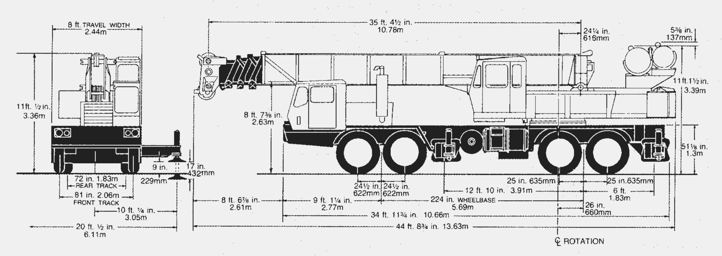
TURNING RADIUS 41 ft. 9 in. (12.73m) GROUND CLEARANCE 101/2 in. (267mm) (with float removed): TAIL SWING 10 ft. (3.05m) - Counterweight in travel position TAIL SWING 12 ft. (3.66m) - Counterweight in working position
