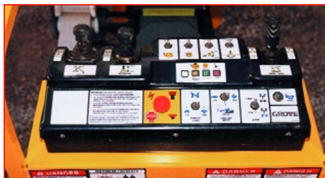
Upper control station features "user friendly" layout
