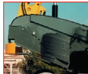
Interactive counter-weight system covers range of boom angles
