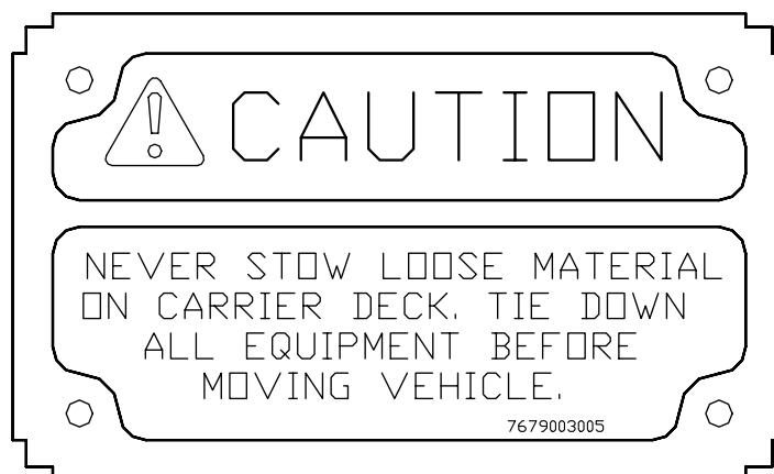
Item No. 25 – Caution Loose Material Stowage
