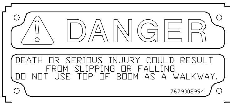
Item No. 1 – Danger Boom Not A Walkway
