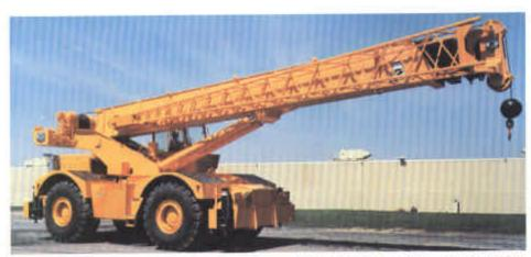
The "SwingAway" lattice boom extension stows laterally along side the boombase section and swings easily into working position to provide 121 (36.9m) tip height with the standard boom and 147' (44.8m) tip height with the optional boom.
