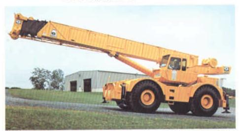
In addition to excellent mobility on all types of fermin, the RT75S leatures low overall height, low center of gravity, excellent ground clearance and a GVW of approximately 74,000 bs. [33 566kg]
