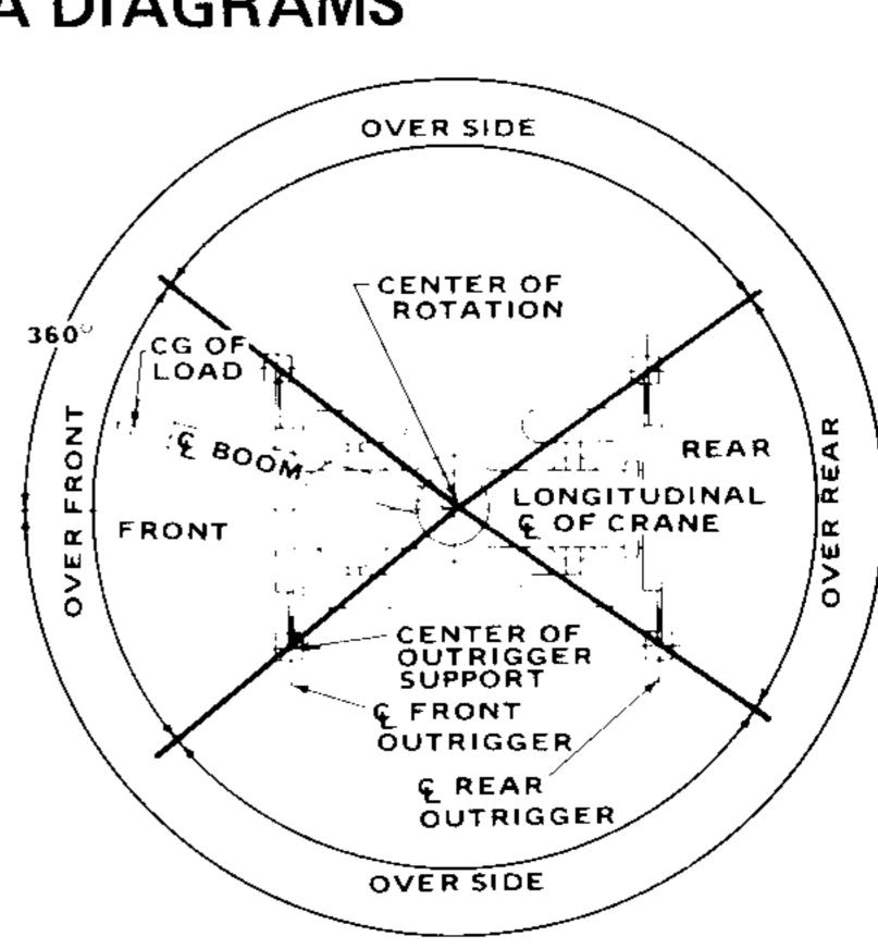
NOTE: BOLD LINES DETERMINE THE LIMITING POSITION OF ANY LOAD FOR OPERATION WITHIN WORKING AREAS INDICATED.
