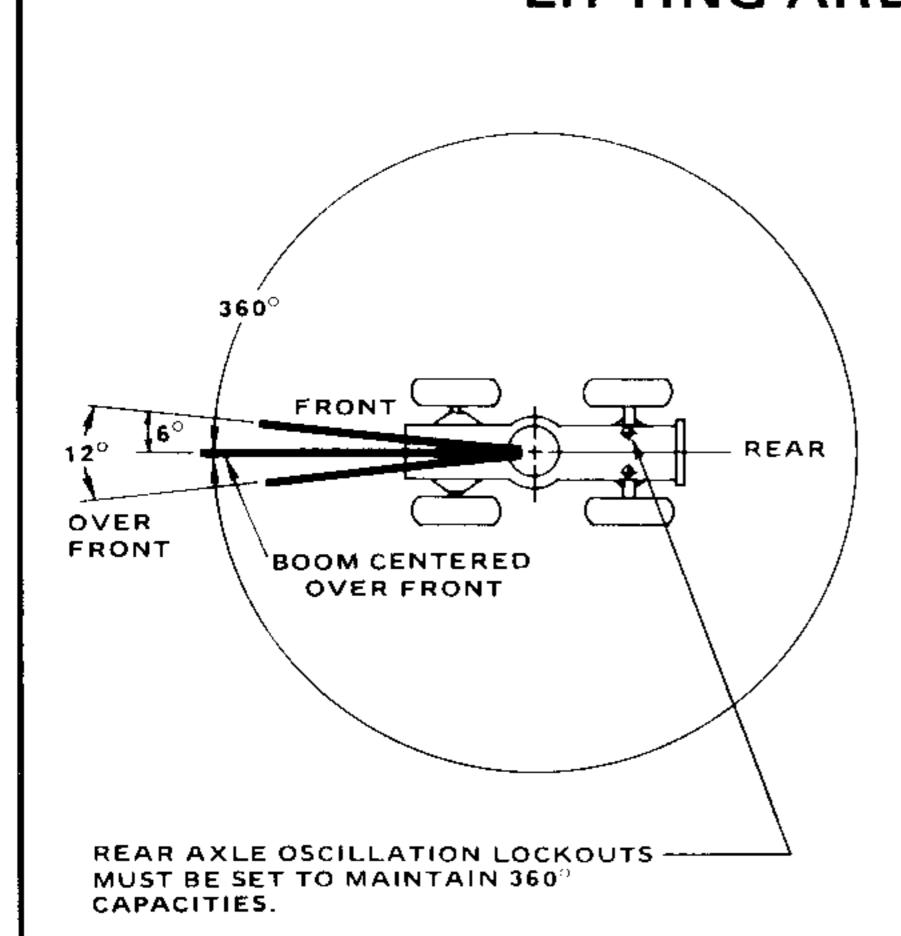
NOTE: BOLD LINES DETERMINE THE LIMITING POSITION OF ANY LOAD FOR OPERATION WITHIN ANY WORKING AREAS INDICATED.
