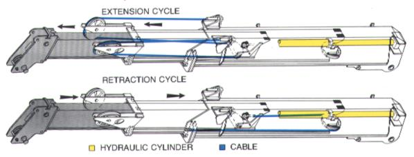
EXTENSION CYCLE – As the mid-section is extended by the telescope cylinder, the fly section is pulled out of the mid-section in direct proportion by a ⅓ in. (22mm) cable. The extension cable has a safety factor of 3.5 to 1 (6 to 1 with international version and 1⅓ in. (29mm) dia. cable) and is attached with threaded connections at base section and retained on either side of the sheave segment by swaged collars. This prevents the boom from retracting should the cable break.
