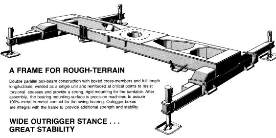
Telescoping beam and jack outriggers have a spread of 17 ft. (5.2m) which provides a nearly square stance for outstanding stability throughout the 360° lifting range. Jacks have a vertical stroke of 21 in. (533mm) and are equipped with integral holding valves. The exclusive Grove Spin-lock†, which permits the jack to be locked mechanically in any position, is available as optional equipment.
