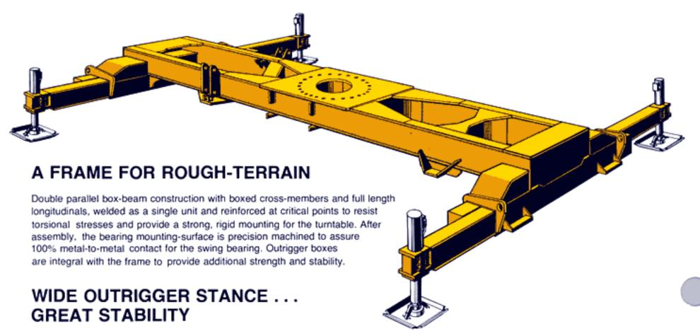
Telescoping beam and jack outriggers have a spread of 17 ft. (5.2m) which provides a nearly square stance for outstanding stability throughout the 360° lifting range. Jacks have a vertical stroke of 21 in. (533mm) and are equipped with integral holding valves. The exclusive Grove Spin-lock†, which permits the jack to be locked mechanically in any position, is available as optional equipment.
