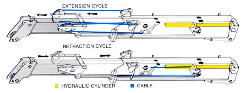
the telescope cylinder, the fly section is extended by the telescope cylinder, the fly section is pulled out of the mid-section in direct proportion by a % in. (22mm) cable. The extension cable has a safety factor of 3.5 to 1 (6 to 1 with international version and 1% in. (29mm) dia. cable) and is attached with threaded connections at base section and retained on either side of the sheave segment by swaged collars. This prevents the boom from retracting should the cable break.
