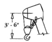
DIMENSIONS ARE FOR LARGEST GROVE FURNISHED HOOK BLOCK AND HEADACHE BALL, WITH ANTI-TWO BLOCK ACTIVATED.
