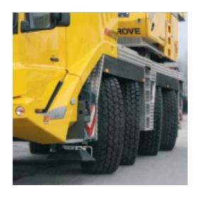
Other systems, where one or more "dead weight" hanging axles remain fixed – lead to higher axle loads, driveline maintenance problems, increased ground pressure and tire wall stress. All-wheel steer enables a fully laden crane to distribute weight evenly across all axles.
