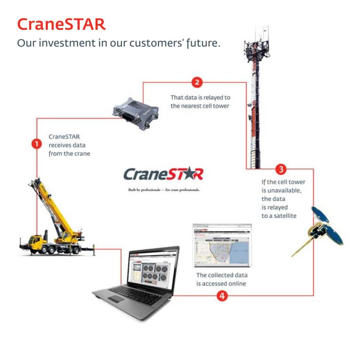
Manitowoc CraneSTAR makes it easier for crane owners to monitor and maintain their equipment. CraneSTAR is the most extensive and innovative OEM-produced crane asset management system available. With its flexible, dual-mode communications capability, GPS and data monitoring and diagnostics, CraneSTAR gives customers near-real-time crane fleet information, no matter where in the world a crane is working.
