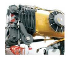
This leads to an intrinsically stronger system. In addition to less weight, a larger cross section area can be used, giving greater lifting capacity at all radii.
