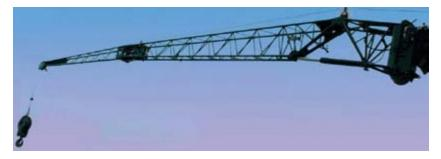
These jibs can also be conveniently stowed alongside the boom for secure road travel.
