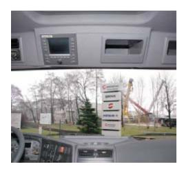
Carrier operations such as suspension and MEGATRAK<sup>TM</sup> controls, differentials and steering modes will be controlled via ECOS as well. The functions can be operated via the screen which replaces the switches usually installed in the middle console of the carrier cab.
