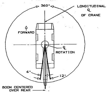
BOLD LINES DETERMINE THE LIMITING POSITION OF ANY LOAD FOR OPERATION WITHIN WORKING AREAS INDICATED WORKING AREA DIAGRAM
