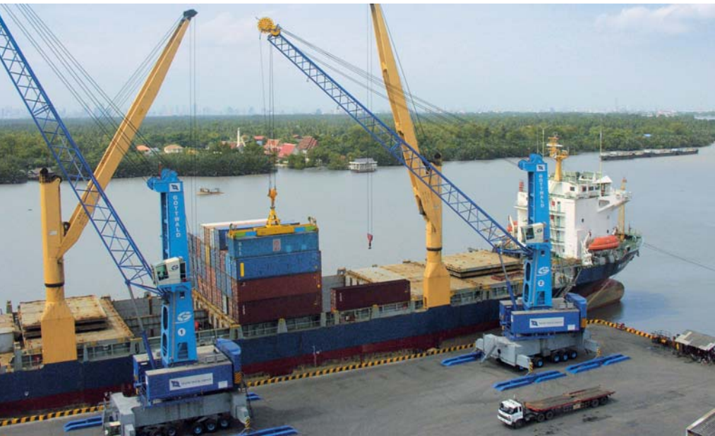
HMK 260 EG in Immingham, UK: the field-tested H-shaped stabiliser arrangement enables the crane to operate even in areas with a minimum of working space
