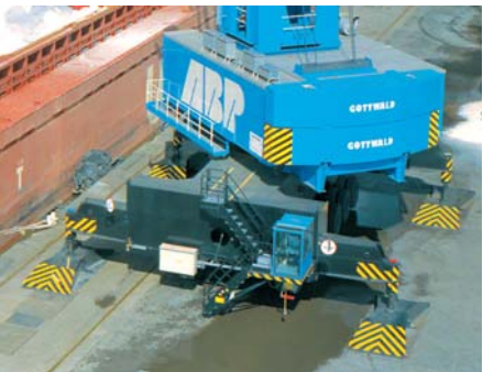
HMK 260 EG in Immingham, UK: the field-tested H-shaped stabiliser arrangement enables the crane to operate even in areas with a minimum of working space
