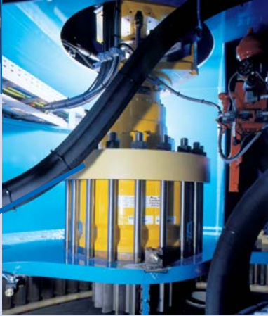
Modular designed slewing gear drive unit
