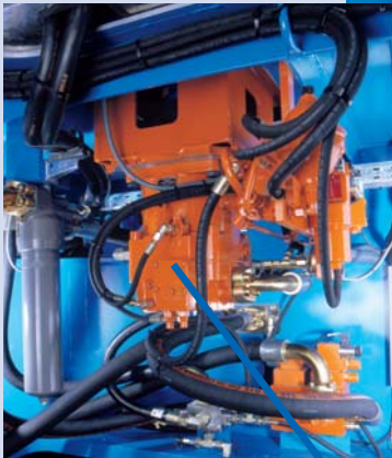
Hydraulic unit driven by an AC motor
