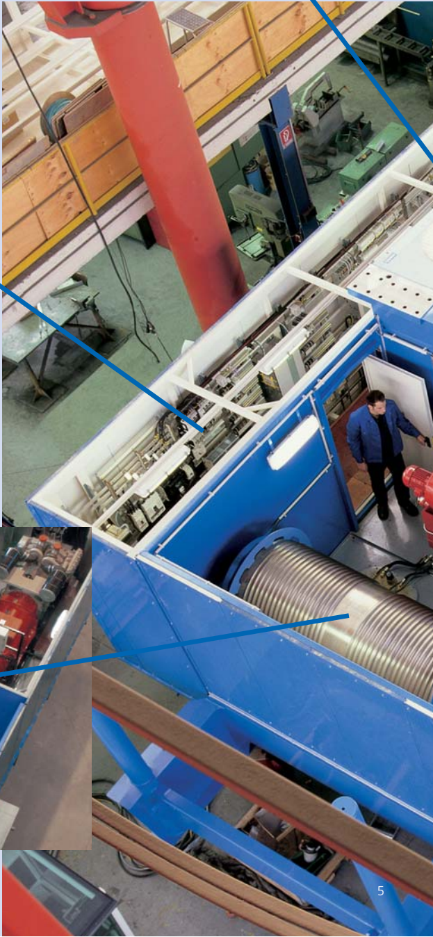
Superstructure with individual rooms, designed as modules
