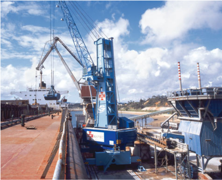
HMK 170 EG handling fertilizer at Sapeç, Portugal: the field-tested H-shaped stabiliser arrangement enables the crane to operate even in areas with a minimum of working space
