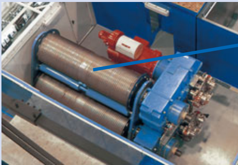
Two hoists for 4-rope HMK 170 EG
