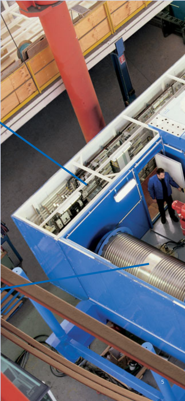
Superstructure with individual rooms, designed as modules
