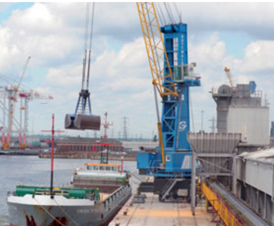
HMK 170 EG handling bulk material, such as scrap and agribulk, at the Port of Southampton, United Kingdom
