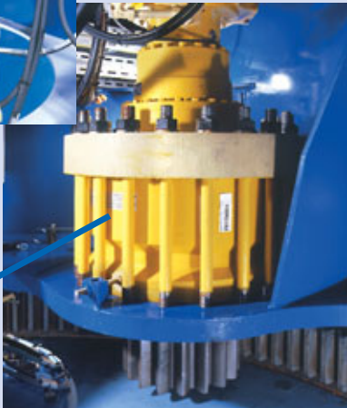
Modular designed slewing gear drive unit
