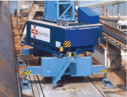
HMK 170 EG handling fertilizer at Sapeç, Portugal: the field-tested H-shaped stabiliser arrangement enables the crane to operate even in areas with a minimum of working space
