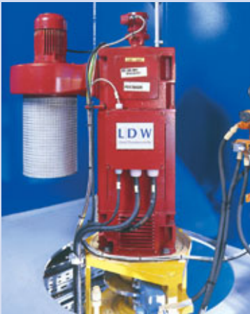
Modular designed slewing gear drive unit
