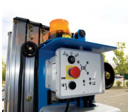
Operational Warning Light
