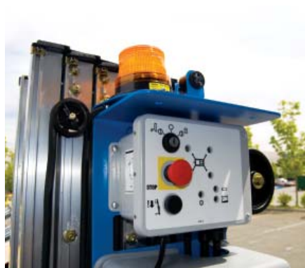
Operational Warning Light
