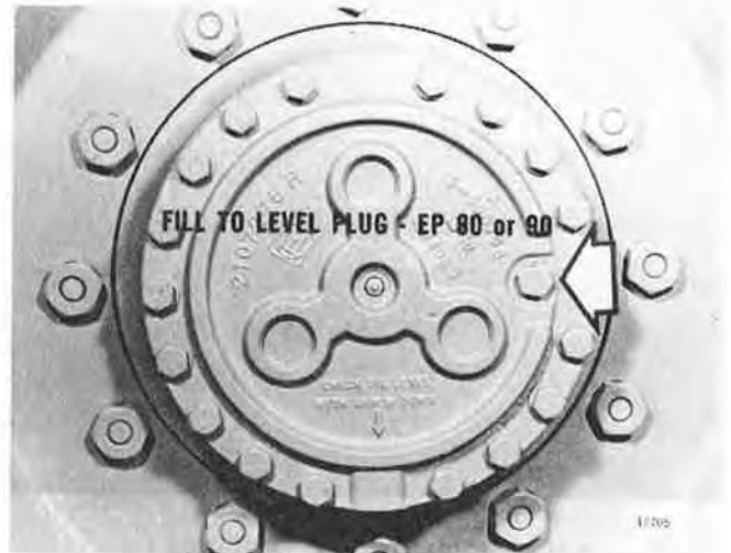
Figure 73 AXLE PLANETARY DRIVE LEVEL PLUG (CLARK DS-13311)
