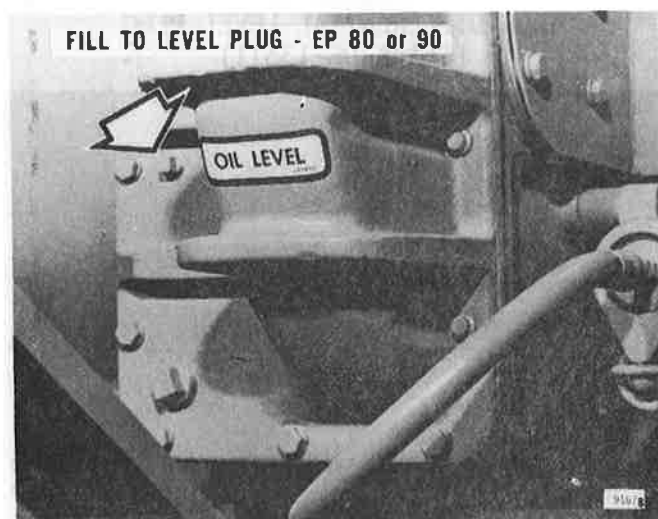
Figure 78 HOIST GEAR CASE LEVEL PLUG
