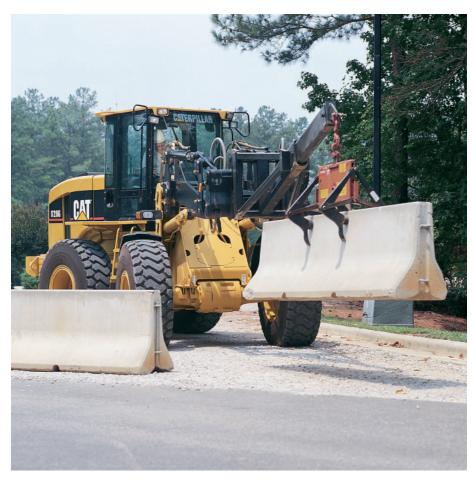
**Auxiliary Hydraulics.** Optional 3rd and 4th function hydraulics are available for use with tools that require hydraulic
