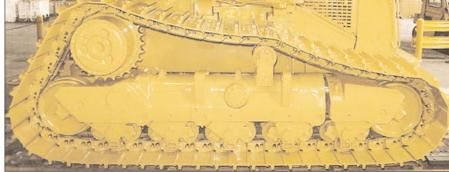
Final drives, steering clutches and brakes relieved of all vertical ground contact shock loads, and roller frame alignment loads – extend power train component life.
