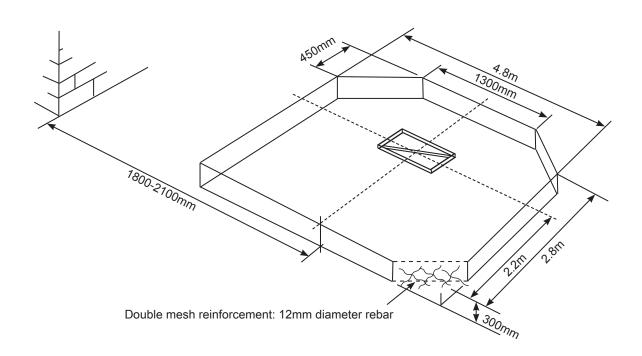
Verify hoist dimensions prior to the foundation design.
