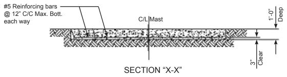
Note: Minimum soil bearing pressure required to be 3,000 PSF
