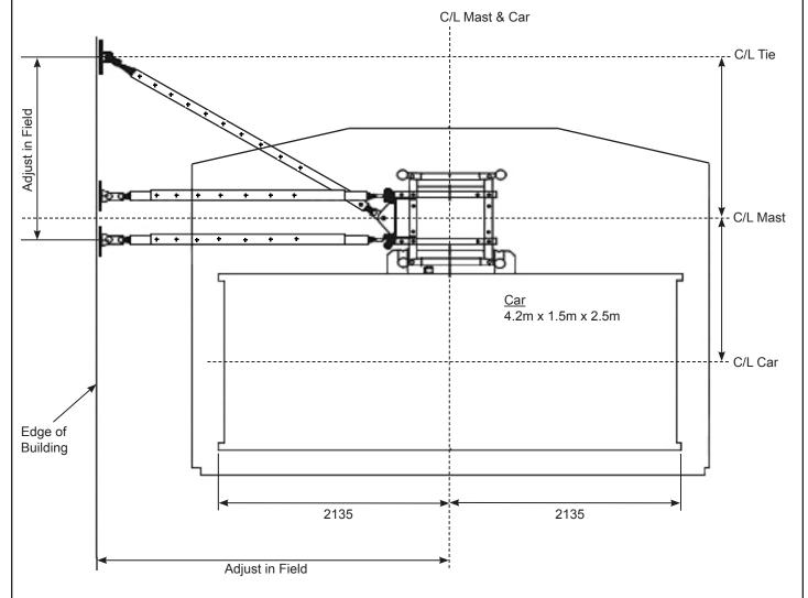
Note: All hoist cages are designed and built in conformance with CAN/CSA-Z185-M87 local safety code. All sizes and dimensions are subject to change at any time without notice and must be verified by a local certified engineer. Any changes or modifications should be consulted with AVRO Hoist Co.
