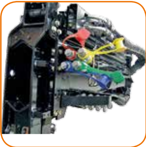
Quick-release couplings for quick tool changes.
