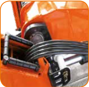
Internal hose routing, good protection for hoses.
