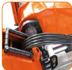
Internal hose routing, good protection for hoses.
