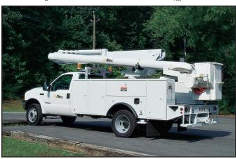
Low stow feature, low center of gravity and low travel height offers operator easy platform access, a stable driving unit and the ability to maneuver in low overhead areas.
