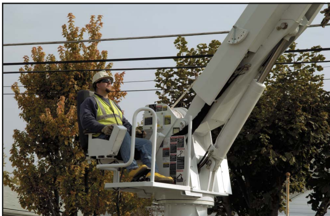
Altec Opti-View® Control Seat increases operator comfort and provides a full view of the work area.
