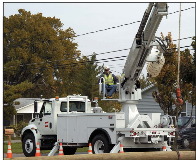
Altec Opti-View® Control Seat increases operator comfort and provides a full view of the work area.
