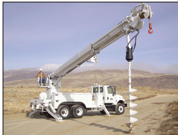
Altec OptiView® Riding Seat Provides Clear View of Work Zone
