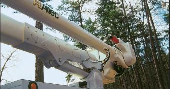
Automatic upper boom stow system reduces setup and stow times
