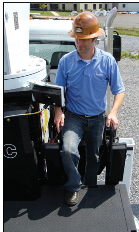
Walk Through Control Stations
